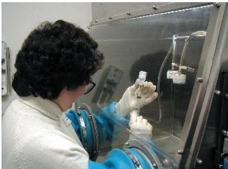
**Industrial hygiene air monitoring performed on an operator doing drug reconstitution (a pharmacy operation) in an isolator. Note air monitors on the shoulder of the operator and inside the isolator**
