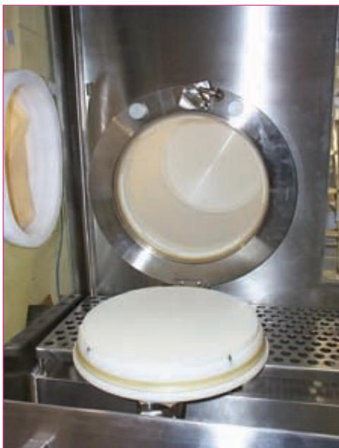
View from inside an isolator: open RTP looking into a Beta Canister (picture provided courtesy Hosokawa Containment).
