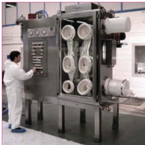
Barrier Isolator showing RTP with Beta Canister fitted (top right) and Bagging Port (bottom right) (picture provided courtesy Hosokawa Containment).
